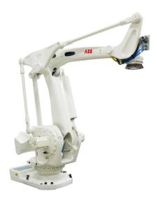
The 4-axis robot can move and rotate large and heavy products at high speeds, and with the utmost care. Its compact design makes it ideal for fitting into existing lines.
