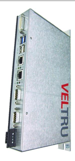
The VELTRU C10 Motion Controller offers a flexible platform for entire automation projects including robotics. The CODESYS V3 based Soft PLC ensures that developers, commissioning and field service engineers are familiar with the system after short training period. VELTRU software libraries include Motion Control, queuing and sorting of parts, machine vision connection, alarm handling and data management.
