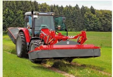
**SAFE TRANSPORT**The RADON 310 FZ achieves an overall lift travel of 490 mm.
