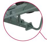
The rotors are stored in special pockets during transport and thus relieve the load on the hinge points and support arms.
