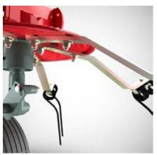
The tine arms are made of tough, galvanised flat steel bar, which allows a wide contact surface between tine and rotor plate. This ensures very good power transmission even under the harshest of working conditions. The forces are optimally absorbed whenever the ground is uneven.
