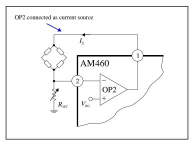
Figure 5: Connecting up a constant current source
