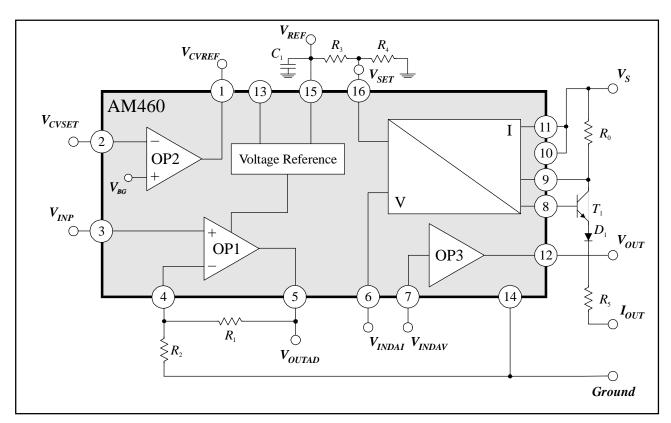
Figure 2: Block diagram of AM460 with external components (3-wire circuit for current output)
