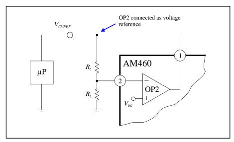
Figure 6: Connecting up a voltage reference
