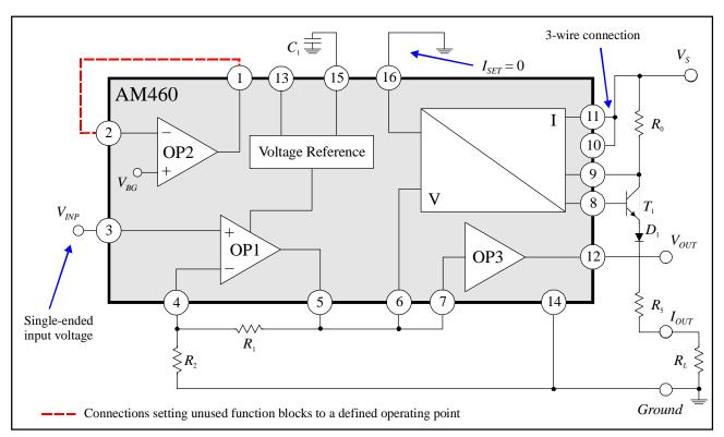
Figure 7: Typical application for input signals referenced to ground
