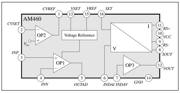
Figure 9: Block diagram of AM460
