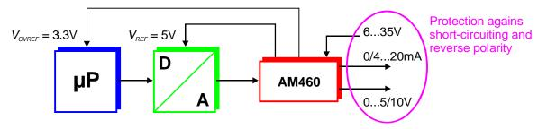
Figure 12: Complex configuration as a peripheral processor IC
