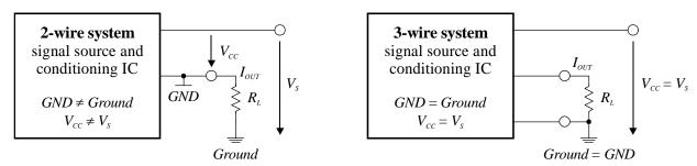
Figure 3: Difference between 2- and 3-wire operation
