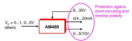
*Figure 11:* Application for input signals referenced to ground (protected output stage, impedance converter etc.)
