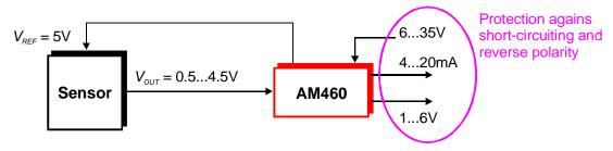
Figure 13: Conversion of a 0.5...4.5V sensor signal
