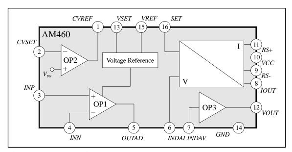
Figure 1: Block diagram of AM460
