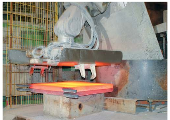
Gripper system for CU: G=650 kg, T=700° C
