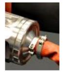
Camera container with polycarbonate front glass and sea water tight hoses on the back to furnish cabling. The camera is installed prior to sealing the housing and operation of camera is by remote control signals ( discrete Remote On, Software etc )
