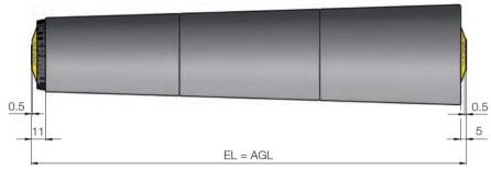
Dimensions for tapered elements on zinc-plated steel tube with two grooves
