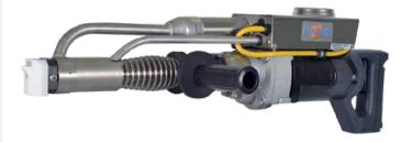
R - SB 50 is a powerful extruder indispensable for jobs that require a high output of extruded material. R-SB 50 is suitable for joining linings and geo-textiles, sheets, thick pipes and for all those welds that are required to resist to continuous stress. During the welding phase the extruder is very smooth and handy.
