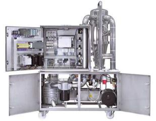
The air unit and the controls are installed in the machine housing, separated from the product area.
