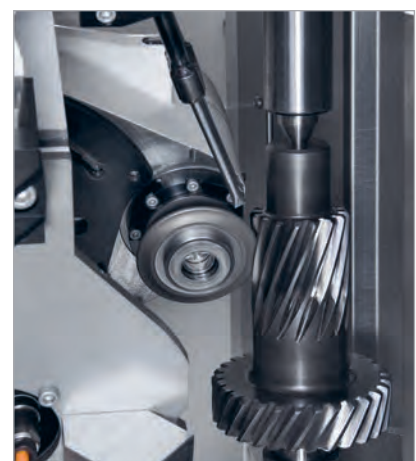
Profile grinding with profile grinding head
