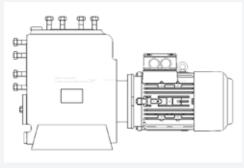
VAC 4001 in close-coupled design with electric motor 5.5 kW at 2850 RPM.
