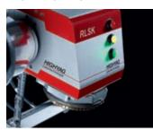
The free focus positioning in the three-dimensional working area of the RLSK from HIGHYAG enables "welding on the fly" during the robot motion.
