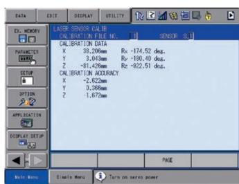
Monitor Lasersensor calibration
