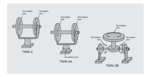
With this function several external axes can be interconnected to one unit. This unit can be managed and programmed similar like one station or base, even though several motors have to be driven and controlled.
