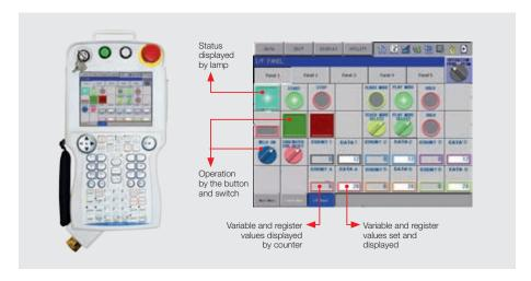
The IF panel enables the possibilty to set up a virtual operation panel within the programming pendant. Frequently used switches, variables or status indicators can be individually arranged and clearly displayed. An existing IF panel which has been set up once can be copied to other controller by uploading configuration file.
