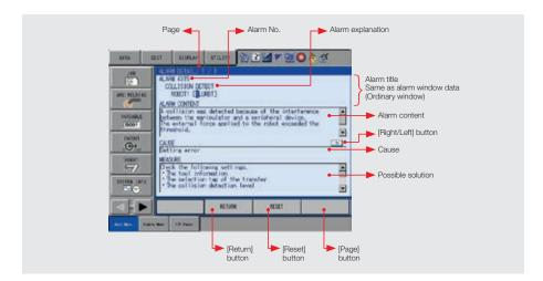
This function simplifies specific diagnostic and fixing of occuring alarms, which are sorted by frequency. Contents, causes and recommendations for fixing the alarms are displayed.
