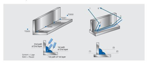
Recording and reproduction of different kinds of paths during multi-layer welding. In the first layer arc sensing will compensate the offsets between taught and current positions with ComArc or MotoEyeLT.
