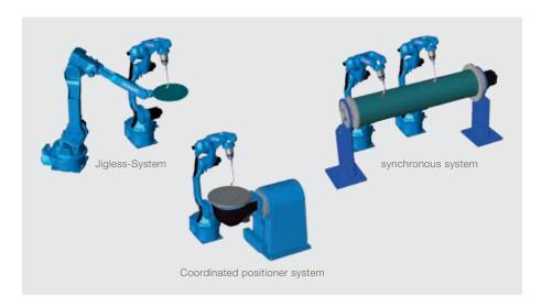
The current controller generation for DX200 is able to manage and control up to 8 robots plus 24 external axis.
