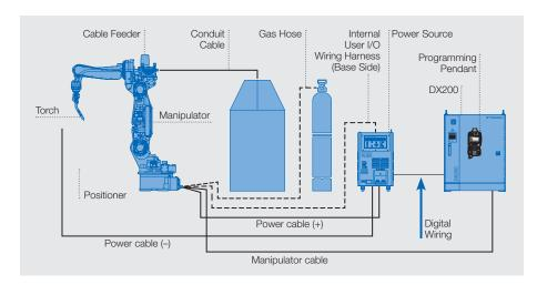
This function enables the communication between robot controller and welding power source by digital interface.
