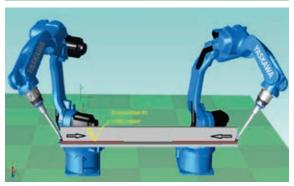
Both robots repeat their program range. At the saved error position, the interrupted robot carries out ignition and can complete the missing weld seam.
