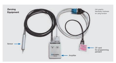
With the zeroing sensor it is possible to quickly restore the home position (absolute data) from your robot or external axis, for example after loss of absolute data.
