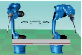
Once a fault has been detected, both robots move to a freely programmable service position.
