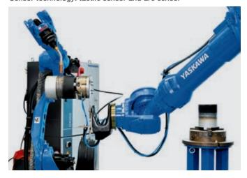
MAG welding on various housing components and subassemblies ES165 with MA1800 Sensor technology: tactile sensor and through-the-arc sensor
