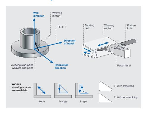
The "hover weaving function" is special weaving mode for applications in which robot positions for start-/end-points are the same: During process robot does not move on a trace!.
