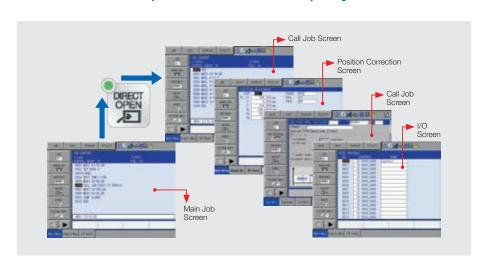
The "direct open" button enables direct access to additional information for each instruction line where they are available: For example job contents in CALL JOB instruction, detailed display of welding or weaving files, input/output screen etc.
