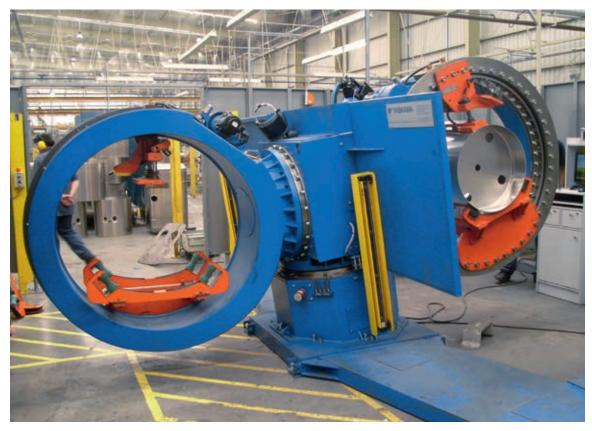
Special design: 5-axis positioning table with steady rest system for machining the end faces of long work pieces, in this case fuel tanks for trucks: welding of cover/bottom with tank casing
