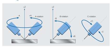
A multi layer design which is created once can be repeated at any position in the cell. The programming works in a special tool coordinate system which corresponds to "Euler angles" where the "alpha angle" means forehand/ backhand welding and the "beta angle" equals torch orientation in the groove.
