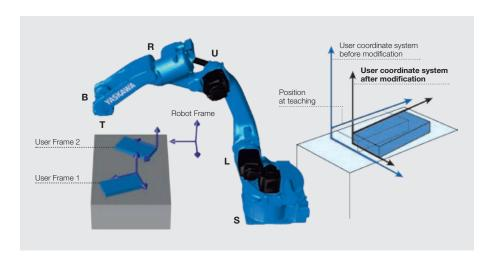
Robots usually store their taught positions in ("standard") pulse jobs where encoder data for each axis are registered. The relative job function offers the possibility to store all positions as xyz data "in relation" to any cartesian coordinate system, like user frame, base frame etc. Relative jobs can be generated when new job will be created or later on by conversion of existing standard job.
