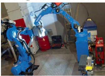
MAG welding on bulk material containers MH400 with MH50-30 Sensor technology: vision system, MOTOSense SeamFinder and tactile sensor
