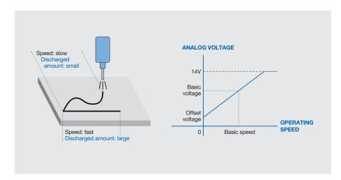
This online-function generates an analogue voltage during the process. Its height is related to robot's real speed. Resolution and pitch of this characteristic are configurable. Common applications you will find in control of bonding or sealing guns. But it can be also used for arc welding, when parameter must be adapted according to "heat input per unit length of weld".
