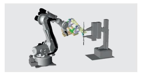
Any application where handling robot must manipulate work piece with devices like press brake, stationary torch or spot gun (left picture) requires this function: it enables the creation of an external TCP in addition to tool centre point of robot. Interpolated movements around this external TCP will be possible now.
