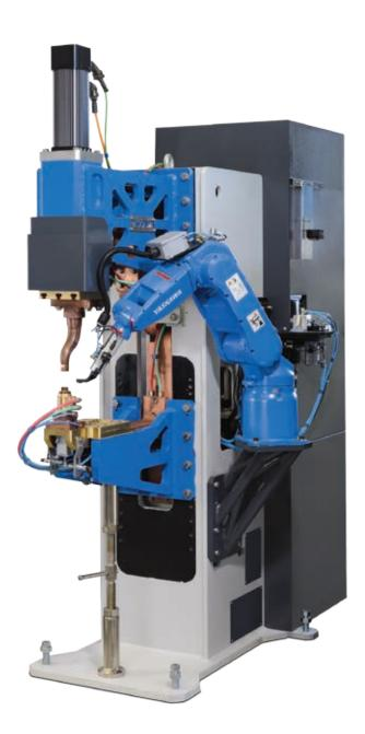
The nut welding machine is the new machine designed and manufactured
