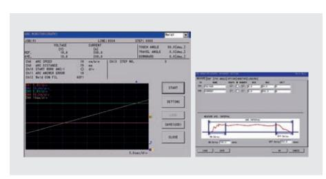
The Graphical Arc monitoring function samples the arc-welding related data and shows them on the programming pendant as a graph and numeric values. The mean value of the last welding is displayed.
