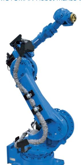
Laser technology is regarded as a driver of innovation in a wide range of applications, such as welding, cutting, build-up welding or marking, and opens up new ways of boosting efficiency. In order to make robotic laser applications even more effective and economical, YASKAWA has developed a new robot the MOTOMAN MC2000 II - that features intelligent interfaces with laser scanners from leading manufacturers, enabling it to exploit its potential to the full.
