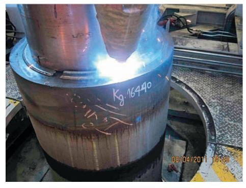
Example for multi layer welding on electrodes for ESR process: Variable layer design for hardfacing and seam welding
