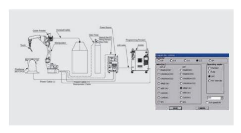
The WELDCOM function serves as a digital interface that communicates via Ethernet with an arc welding power source.
