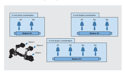
YASKAWA systems can operate simultaneously and fully synchronized with 2 (Twin), 3 (Triple) or 4 (Quad) robots at one rotation axis.
