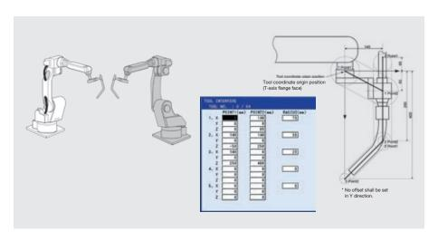
This function checks the interference among manipulator arms and tools in the system consisting of one controller and multiple manipulators.
