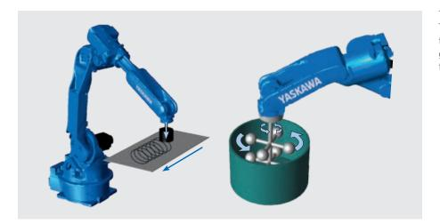
This function continuously rotates the T-axis a plural number of turns. Although the rotation angle of the T-axis is generally limited within ±360 degrees, this function allows it to rotate endlessly.
