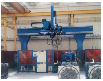
Three-axis gantry system for welding industrial heat exchangers
