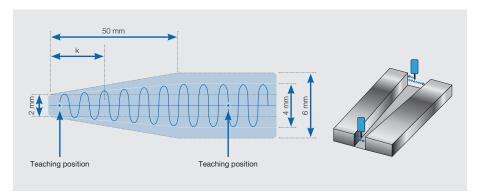
This function can be used to compensate variable conditions in a welding groove by continuous adapting of weaving parameter and speed.
