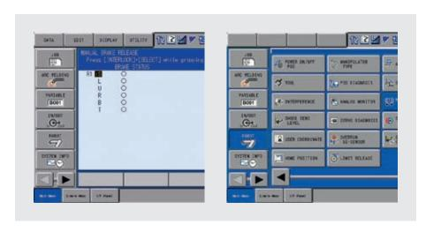
The manual brake release function allows specific brake release by programming pendant for each servo motor in the system: Robot axis as well as external axis.
