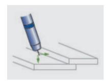
Simplest, but most inexpensive and service-proven method of static component measurement, e.g. search for start point: using search runs until component contact is achieved, differences between the original component and the current component can be detected and program points shifted accordingly. Switching contact is carried out by means of an electric short circuit (search voltage on wire or gas nozzle) or mechanical sensor.
