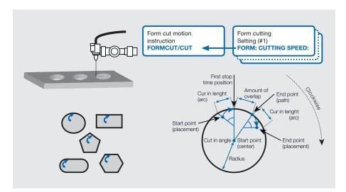
The form cutting function allows a quick and comfortable access to simple geometric figures which are stored in preconfigured files.
