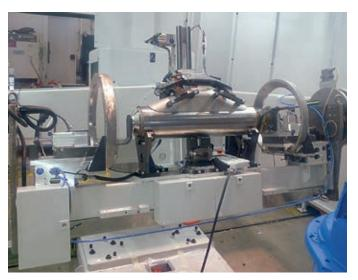
Jig construction in MSG welding cell for flowmeters (pressure vessels)
