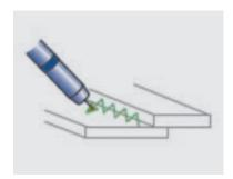
Seam tracking system that uses a shunt to detect the changes in current strength in the arc as the length of free wire changes during weaving. The resulting differences from the taught values for this seam form the basis for a correction of the welding path. Unlike with "static" measurement, it is possible in this case to respond to discrepancies that arise during the process as a result of shrinkage and distortion.
