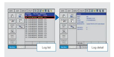
During operation all relevant events (p.e. job changings or switching the operating mode) are registered and can be displayed for diagnostic purposes.
