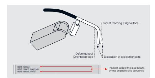
This "mini" program inside the controller converts robot programs to another tool. This would be required for example in case of using another kind of torch with a different tool-centre-point as the original torch for which the program was created.
