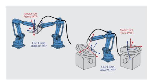
The "Master Tool User Frame" is a special function for jigless systems and coordinated motion systems. This type of user coordinate system is related to master tool frame of "master" robot or station axis.
