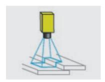
MotoSight2D is a fully-integrated hardware/software package for the 2D view. It enables the robot controller to communicate with the Cognex In-Sight sensor devices. MotoSight2D includes a teach pendant application that is used for the direct assignment of supported visualization device results to robot variables for use in robot programs. Recorded images and visualization graphics appear directly on the display screen of the teach pendant.
