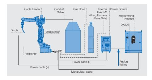
With the ARC-Anlag Basic function the robot controller and the welding power source can communicate by digital interface.
