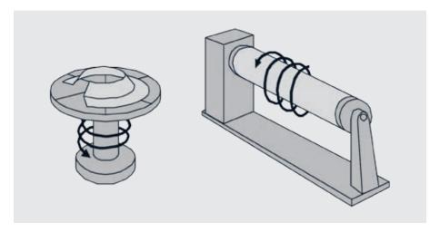
This function continuously rotates the external axis a plural number of turns. Although the rotation angle of the external axis is generally limited within ±360 degrees, this function allows it to rotate endlessly.
