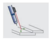
YASKAWA product: one-dimensional laser, diffuse reflective sensors, search routines such as those described above, but non-contact. Steps on the component are detected by means of the surge in intensity of the reflected laser beam.
