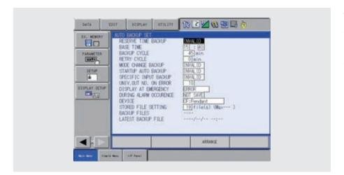
At regular intervals the automatic backup function creates a backup file containing all current controller data. In case of unexpected problems the latest controller state can be restored at any time.
