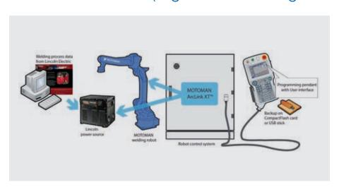
This software, based on Ethernet communication, enables an exclusive operating and controlling of current Lincoln power sources using the YASKAWA programming pendant. Up to four interfaces per controller can be managed. There is no need of additional control elements on the power sources.
