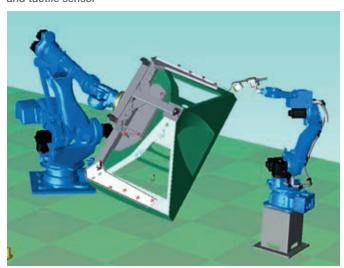
Flexible Multi-Robot system for demonstration, testing and training purposes at the Application Center in Allershausen MH225, 2x MA2010 and turn-tilt positioning table Sensor technology: tactile sensor and arc sensor
