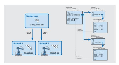
DX controllers can manage up to 8 robots plus 24 external axis. The "independent control function" allows to execute several programmes with different axis group combinations at the same time.
