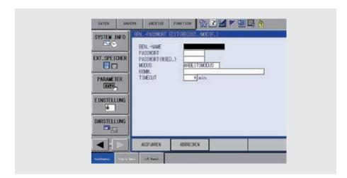
The password protection function helps assure system safety by requiring each user to have a personal authorization registered
