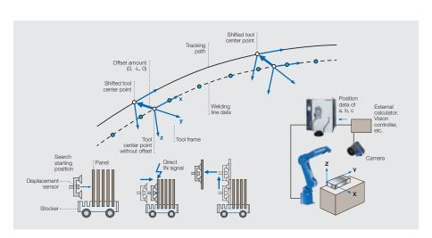
Universal interface for all kinds of analogue sensors. By means of sensor inputs different functions can be realized, for example tracking, speed control and position adjustments.
