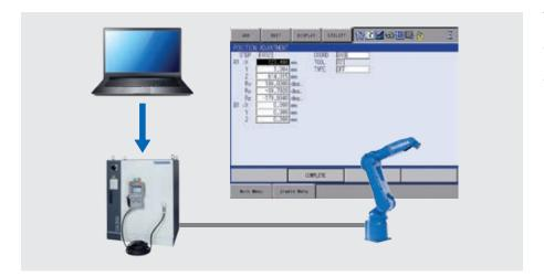
The "teaching point adjustment function" modifies the taught positions by using the numeric keys on the programming pendant without operating the manipulator (offline editing).
