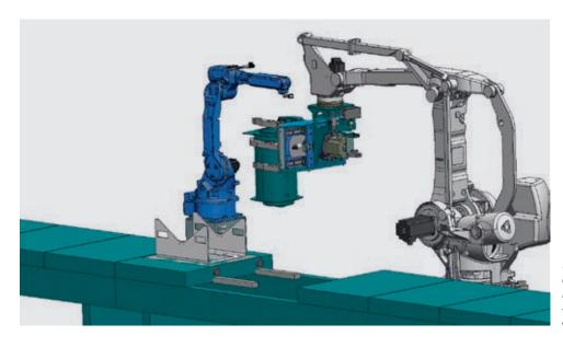
Unmanned MAG welding on large heat exchangers MPL800 with HP20 Sensor technology: tactile sensor and through-the-arc sensor
