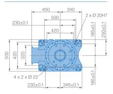
Mounting option: Floor IP Protection: IP54/67
