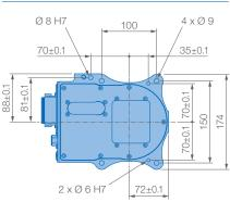
Mounting options: Floor, ceiling, wall, tilt Protection class version YR-1-06VX4-A00 standard: IP67
