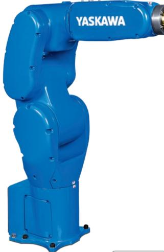
The MOTOMAN GP4 is the smallest 6-axis robot in Yaskawa's GP-series model range and offers high performance for a wide range of applications, such as flexible handling, machine tending and assembly applications, with a payload of up to 4 kg. Providing an outstanding repeatability of  $\pm 0.01$  mm, it is ideally suited for use in the electronics sector as well as for high precision assembly and quality testing applications.
