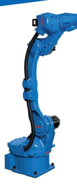
The 6-axis MOTOMAN GP8L is a fast, general-purpose industrial robot with 8 kg payload and a long reach of 1,636 mm.
