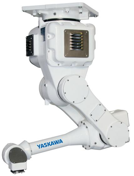
The MOTOMAN MPK2F is a five-axis, high-speed robot that is particularly suitable in the following areas: order-picking, high-speed handling, picking-packing-palletizing and many other handling applications.
