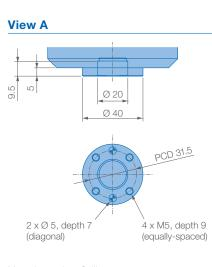
Mounting option: Ceiling Protection class: IP67
