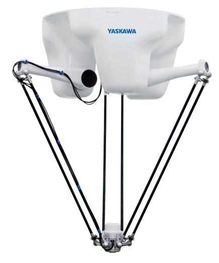
The MOTOMAN MPP3H 4-axis high-speed robot with parallel kinematic system combines the speed of the delta design with a high payload capacity and a large working range. Due to the high torque of the fourth axis, the so-called wrist axis, the MOTOMAN MPP3H moves payloads of up to 3 kg at unprecedented speeds. This delta robot was developed for a wide spectrum of industries, such as food and beverage, pharmaceutical and the automotive sector.
