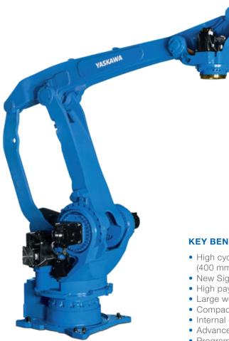
The fast 4-axis MOTOMAN PL190-100 achieves top performance with over 2000 cycles per hour for box, carton and pack palletizing in final packaging and logistics.
