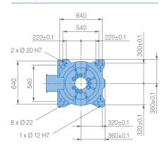
Mounting option: Floor IP Protection: IP54
