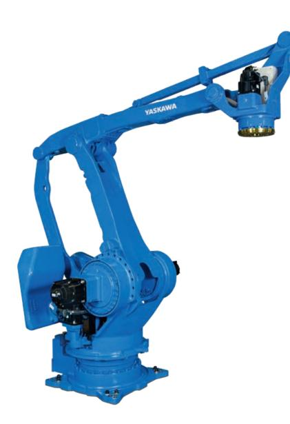
The most powerful 4-axis robot of the PL-series is the MOTOMAN PL800 with a payload of 800 kg. This palletizer offers high performance for box, carton and pack palletizing in versatile end-of-line packaging and logistics applications. The large working range with a maximum reach of 3159 mm and an achievable stacking height of over 2624 mm allows versatile use across all palletizing applications.
