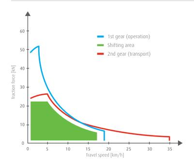
Shift in Motion enables shifting procedures in a moving machine, equipped with a manual transmission that is intended to be shifted at standstill by electro-hydraulically synchronising the drivetrain. This system is particularly suitable for vehicles that often change between transport and operation, i.e. vehicles that require both high tractive effort and a high top speed above 25 kilometres per hour.
