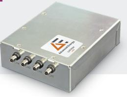
The Luxtron<sup>®</sup> m924 module uses Fluoroptic<sup>®</sup> technology, based on a temperature sensitive phosphorescent sensor attached to the end of an optical fiber. The complete m924 OEM solution consists of the electronics module assembly plus Luxtron probes and accessories. The system provides precise and repeatable in-situ temperature measurements for control of processes involving RF, EMI, magnetic fields and high voltages.
