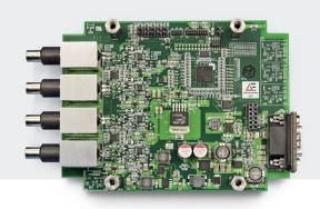
The Luxtron® m924 Utility FOT Module is a cost effective choice for accurate, real-time transformer winding hot spot monitoring. This module is specifically designed for transformer monitoring system providers or transformer manufacturers desiring to add fiber optic temperature measurement capability to their equipment
