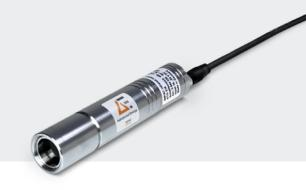
The Impac® KTS 218 and KTG 218 recognizes hot objects located with non-contact monitoring, to trigger a switch process. The switching level can be adjusted via potentiometer and the switch status is indicated by LED.
