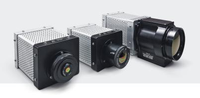
The Mikron® MCL640 is a cost-effective, high performance non-contact infrared imager that produces superior images and temperature measurement (±2°C) for a broad range of process monitoring applications. Designed with advanced maintenance-free electronics and industrial protective packaging, the MCL640 offers unparalleled accuracy for demanding industrial and manufacturing applications with an unmatched array of protective accessories.
