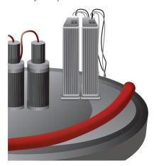
MXE pyrometers mounted side-by-side on tool
