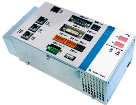
The IPC 221 is an industrial PC with a Celeron1020E processor. It is used to control S-DIAS modules and has various interface connections such as: a VARAN Manager with 2 VARAN Out interfaces. A 7-segment display and 3 status LEDs provide information on the actual status of the CPU directly on the IPC.
