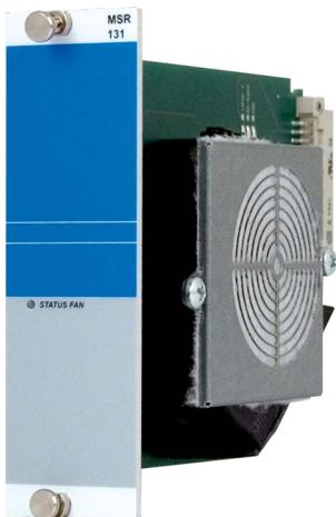
The fan module is an exchangeable unit. Here, a radial fan is mounted on a circuit board. The side intake air is distributed through an air duct in the 19" housing. The fan is activated over the module carrier. To avoid misplugging, a DIN connector (connection to the module carrier) is offset from I/O base or interface module.
