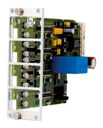
The base module serves as the interface for the insert modules. The base module serves as the interface for the insertable modules; it is addressed over the LVDS bus. In the base module, galvanic isolation is implemented for the analog modules.
