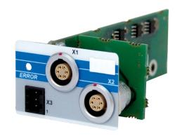
This analog input module is used to record voltages in the range of ±10 V. The module has two channels, each with a short-circuit proof reference voltage of 10 V. In addition, each channel has a 24 V supply voltage.
