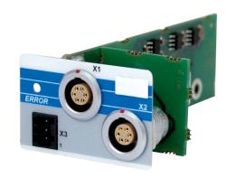
This analog insert module is used to detect currents from 0 to 20 mA. The module has two channels, each with a short-circuit proof reference voltage of 10 V. In addition, each chan-nel has a 24 V supply voltage.
