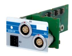
This analog insert module is used to detect temperatures in the range of -200 ... +250 °C (-328 ... +482 °F). A Pt100 resistance thermometer is used as the temperature sen-sor in a 2 or 4-wire configuration. The module has two channels. Additionally, each channel has a switchable 24 V supply voltage.
