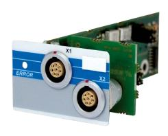
This module has two counter or SSI (Serial Synchronous Interface) inputs. The counters are 32 bits wide and can be used as a counter or frequency meter. The two channels can be configured through the software as counters or an SSI interface. The SSI interface is designed to function as an SSI sensor. Uncoded and Gray encoded sensors are supported.
