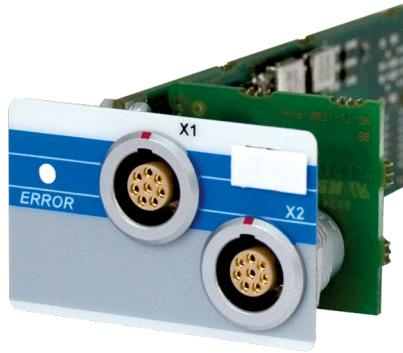
This input module has two independent counter stages for incremental encoder with a RS422 signal. The module provides a 16-bit counter resolution with a maximum input frequency of 125 kHz.
