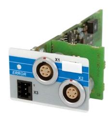
This input module is used to measure the expanding or compression of strain gauges with a Wheatstone bridge. The module has two channels, each with a short-circuit proof excitation voltage of 3.333 V. The measurement range of the Wheatstone bridge is 3 mV/V. Other measuring ranges starting from 1.5 mV/V are available on request. The strain gauges can be connected with 4 or 6-wire technology. Drift correction (zeroing) is Possipble.
