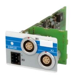
This input module is used to measure the expanding or compression of strain gauges with a Wheatstone bridge. The module has two channels, each with a short-circuit proof excitation voltage of 3.333 V. The measurement range of the Wheatstone bridge is 10 mV/V. Other measuring ranges starting from 1.5 mV/V are available on request. The strain gauges can be connected with 4 or 6-wire technology. Drift correction (zeroing) is possible.
