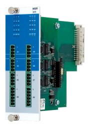
This module has 24 short-circuit proof +24 V/2 A (positive switching) digital outputs, which are back-readable and therefore can also be used as inputs with a +24 V level for reading the signal conditions 0 and 1.
