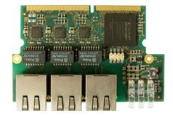
With this expansion card, an analysis tool for the VARAN bus can be added to the C-IPC. The VARAN Analyzer can be operated using the VARAN Service Tool or through an application. The special design allows the expansion card to be easily mounted and secured.
