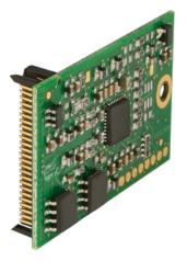
This client board is used to easily equip any periphery device with the VARAN bus. Data can be exchanged over tan alternating buffer and DPRAM.
