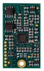
The VEB 012 VARAN client board serves to easily expand all possible peripheral devices with the VARAN bus.
