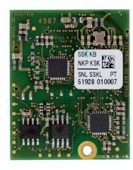
The VEB 013 VARAN client board serves to simply expand all possible peripheral devices with the VARAN bus.
