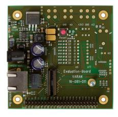
The VARAN VEB 022 demo board provides VARAN users and sensor/actuator manufactures with simple hardware so that they can implement this bus system in their products quickly and easily.
