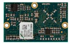
The VARAN Manager board is used to equip all peripheral devices with the VARAN bus as simply as possible. By using the VEB 031 and with minimal external wiring, the peripheral device is expanded over the PCI bus with 2 VARAN Manager interfaces.
