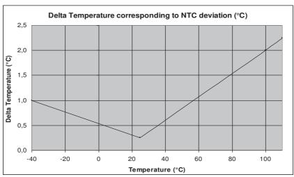
0.1°C tolerance on Resistance Measurement
