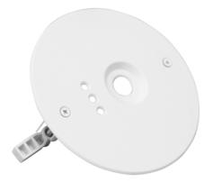
The **RC-1AW** is a one-piece plastic mount intended for recess mounting Brickstream 2Dvideo analytics appliances into ceilings with an unexposed open void. Used in mounting applications where discreet profile is required, the 2Dis inserted into the housing and secured by two attached tension clips. The RC-1AW grips the unexposed portion of the ceiling panel with two swiveling clamps.
