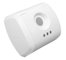
The **SM-1AW** is a two-piece plastic mount intended for surface mounting Brickstream 2D video analytics appliances. Used in mounting applications where no tilt is required, the main housing of the SM-1AW is affixed to the ceiling by four screws (not included). After snapping the 2D into the main housing, the finishing cover is snapped into place leaving only the 2D's lens and status LEDs exposed.
