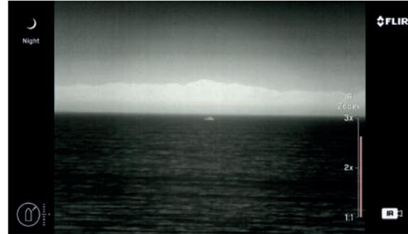
*Recognizing a target means you can verify it as another vessel, as opposed to an island. FLIR uses a 30' outboard boat as a benchmark.*
