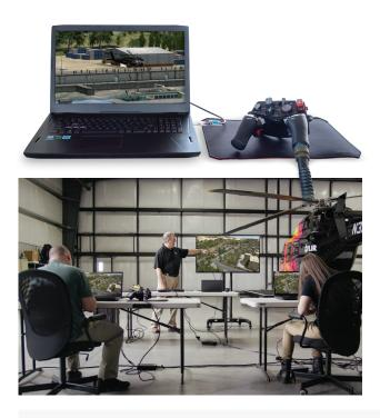
FLIRSIM is a portable, easy to set up and use, all-inclusive system-level training device that provides the functional equivalency of an FAA FTD level 6 simulator for Star SAFIRE 380 family sensor operators.
