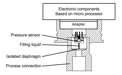
Pressure transmitter includes two functional units:
